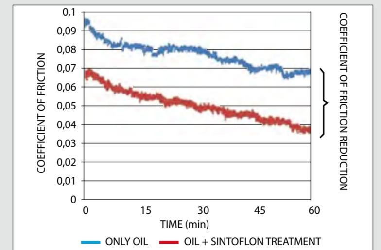
The addition of Protector, in the optimum 10%, significantly reduces the friction coefficient of the coupling, increasing the oil anti-wear properties.
